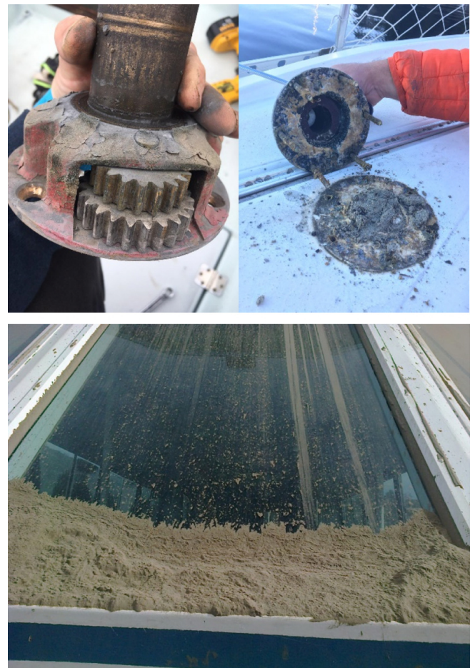
Figure 5: At the top, effects of volcanic ash on motor-sailors at Club Náutico Bariloche ( Lago Nahuel Huapi ) after 2011–2012 Cordón Caulle volcanic eruption. Photos courtesy of Club Náutico Bariloche . Below, deep abrasion on the Catamarán José Julián wind glasses, in Puerto Canoa ( Lago Huechulafquen ), requiring full replacement after the 2015 Calbuco volcanic eruption. Photo courtesy of Catamarán José Julián .
