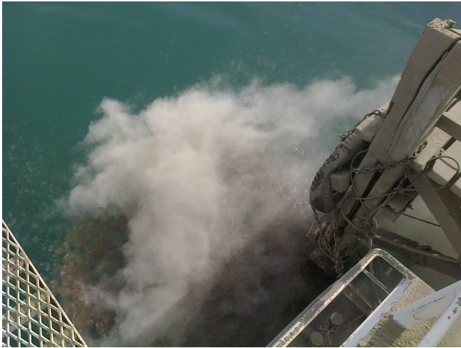
Figure 11: Remobilization of subaqueous ash deposits at Puerto Canoa ( Lago Huechulafquen ) by action of the Catamarán José Julián propellers, many months after the 2015 Calbuco volcanic eruption.
