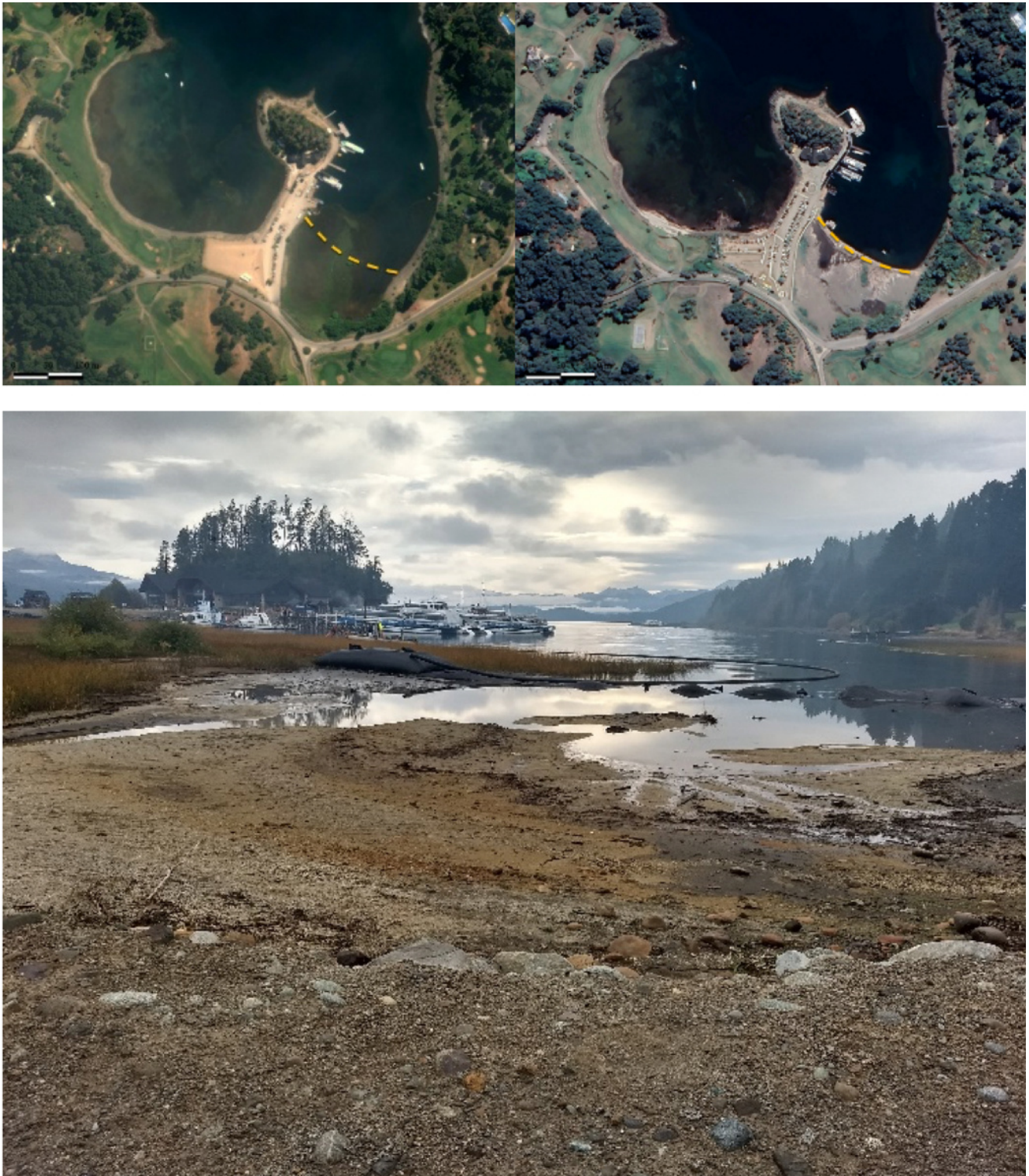
Figure 10: Aerial view of Puerto Pañuelo , before the volcanic eruption (February 2011) at the top left; and ten years later (November 2021) at the top right. The dashed line indicates the position of the gabion wall constructed to retain tephra dredged from the bay since 2011. Below, dredging works in Puerto Pañuelo , many years after the 2011–2012 volcanic eruption, still removing great amounts of settled tephra from the inner basin (May 2019).
