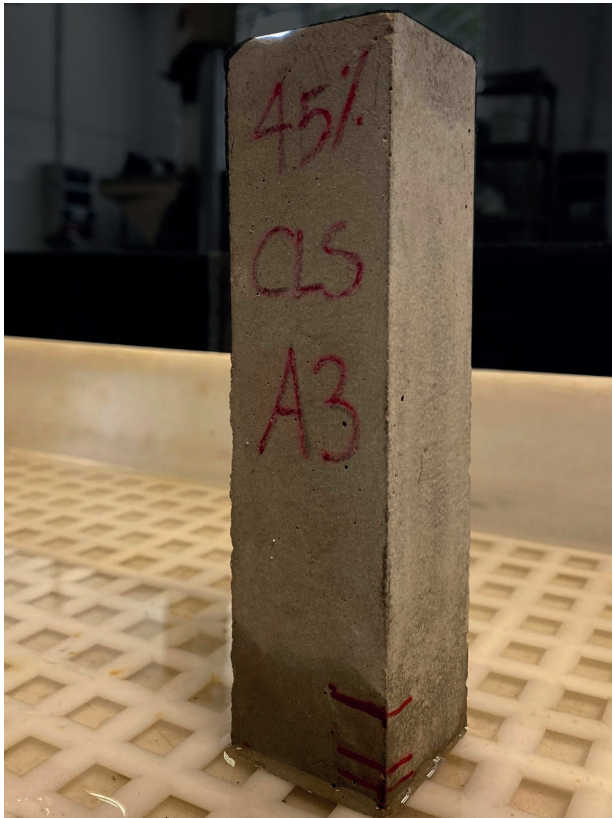
Figure 3 | Absorption test by capillarity.
