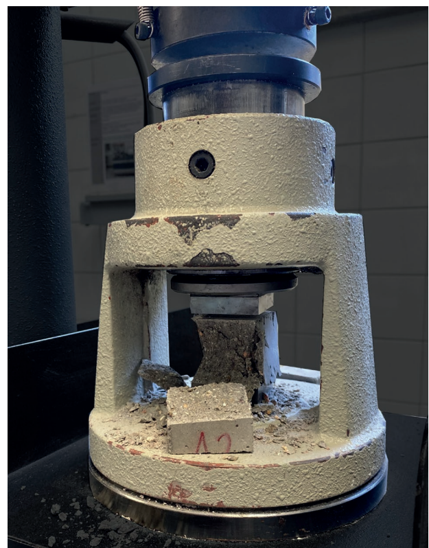
Figure 2 | Flexural and compressive strength.
