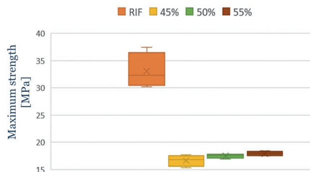
Graph 3 | Results of compressive failure of specimens at 21 days as a function of replacement percentage.
