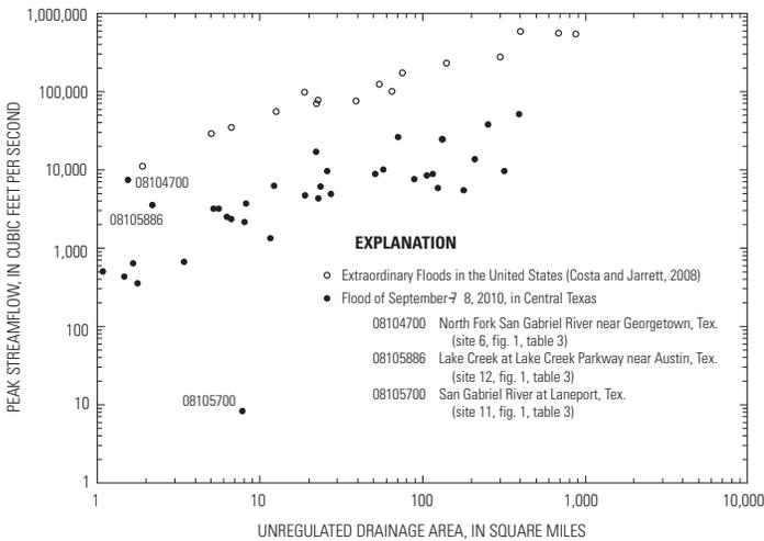
**Figure 6.** Relation between peak streamflow and unregulated drainage area at 35 U.S. Geological Survey streamflow-gaging stations September 7–8, 2010, in Bell, Williamson, and Travis counties and selected flood peaks used to define an envelope of maximum floods documented in the United States by the U.S. Geological Survey.
