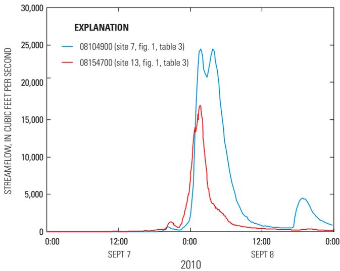
**Figure 5.** Streamflow hydrographs for U.S. Geological Survey streamflow-gaging stations 08104900 South Fork San Gabriel River at Georgetown and 08154700 Bull Creek at Loop 360 near Austin.
