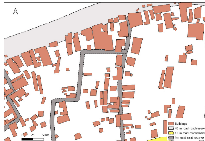
Figure 3: Overlay of buildings and road reserves (note the buildings encroaching on road reserves)
