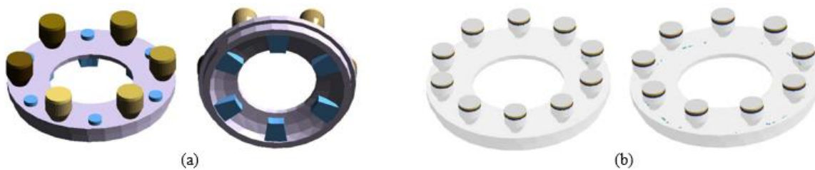
Figure 9. (a) Feeder and chills in cope (left) and drag (right) (b) Shrinkage distribution by autonomous optimization (left) and DOE (right) (Hahn et al. 2010).
