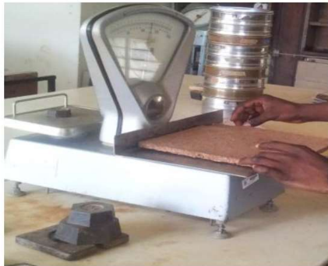
Figure 4. Measurement of the briquette mass on a weighing balance.
