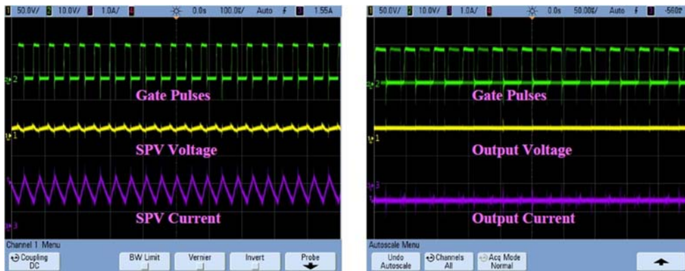
Figure 17. Voltage and current waveforms in a scanned maximum power point training (SMPPT) system with partial shading.
