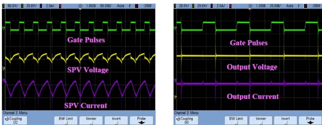
Figure 16. Voltage and current waveforms in a scanned maximum power point training (SMPPT) system without shading.
