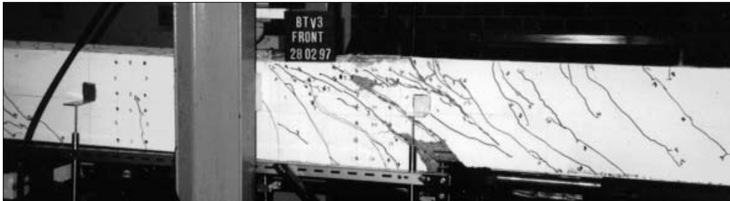
Figure 14b. Computed and observed crack development in the front web (BTV3)
