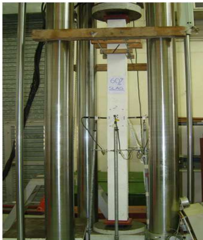
Figure 6. Typical column installed on teh 5000 kN DARTEC testing machine
