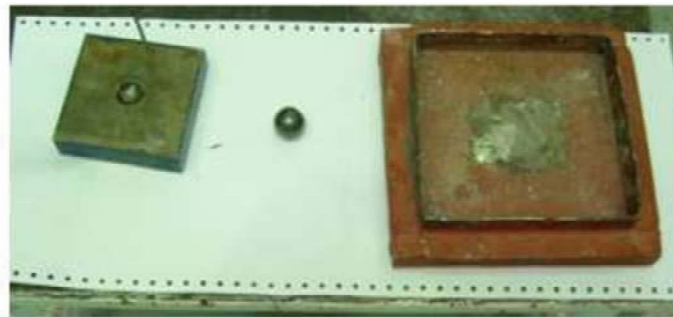
Figure 5. Base plate, ball and cap used at the bottom and top ends of the column
