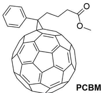
Figure 6a. Chemical structure of phenyl-C61-butyric acid methyl ester (PCBM).
