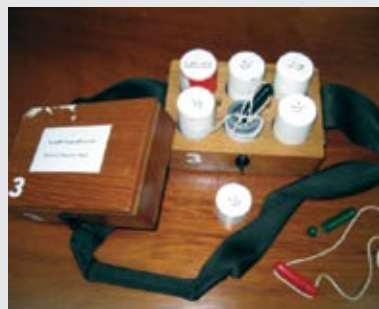
Figure 3: Set of dosimeters in lead pots within wooden box for patients and family members
