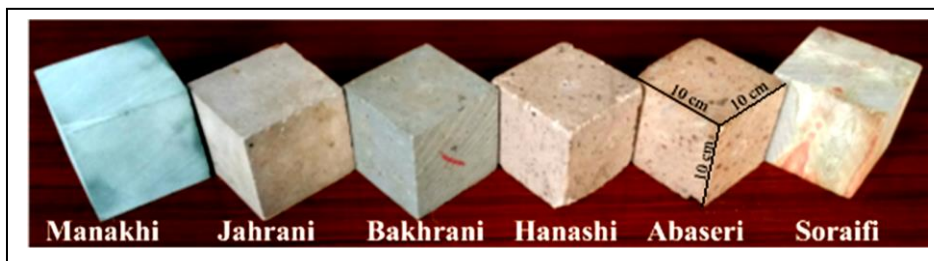
Figure 3. Samples cut into 10×10×10 cm 3 from six quarries used for various tests
