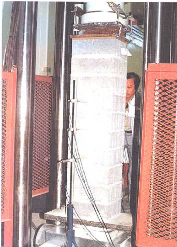
Figure 16. Test of column.
