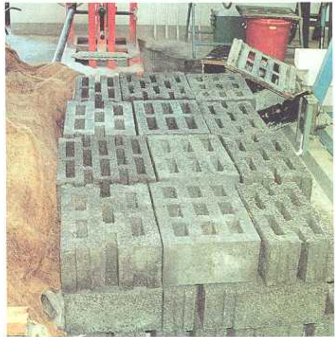
Figure 3. Stack of hollow blocks.
