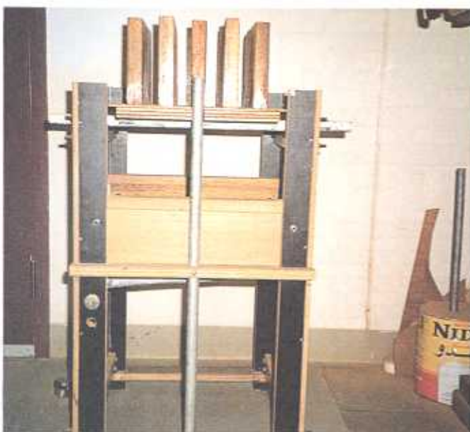
Figure 12. Block-moulding apparatus used in the laboratory
