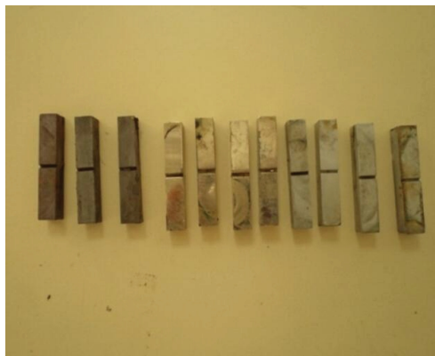
Figure 1. (d) Samples after corroding for 2400 hours
