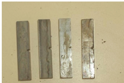
Figure 1. (e) 6 \mu Coated samples of PVD and electroplated samples corroded for 2400 hours
