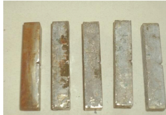
Figure 1. (g) from left to right: uncoated sample of aluminum, 6 \mu Ni coated aluminum, 20 \mu Ni coated aluminum, 40 \mu Ni coated aluminum and 60 \mu Ni coated aluminum after corroding for 2400 hours
