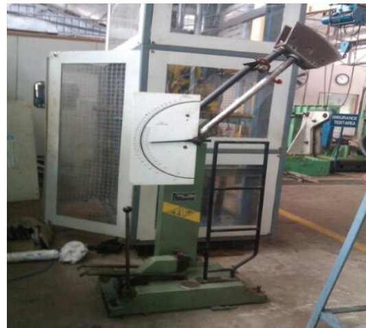
Figure 1. (e) Charpy impact tester
