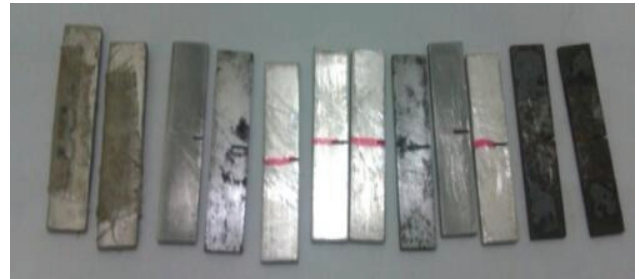
Figure 1. (d) Patched and unpatched samples
