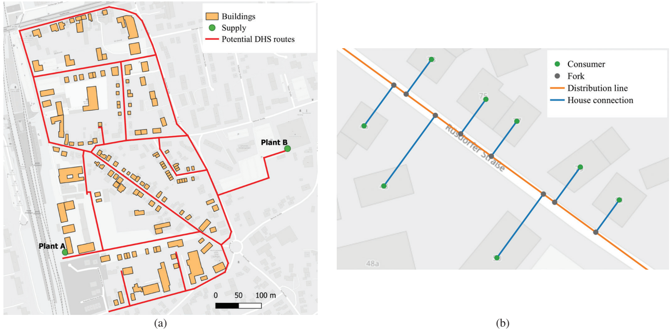
Figure 1: (a) Geometry input of the district planning and optimisation approach. Red: possible district heating routes; orange: considered buildings. (b) Result of the geometry processing and input for the optimisation model builder. Source background map: [41].
