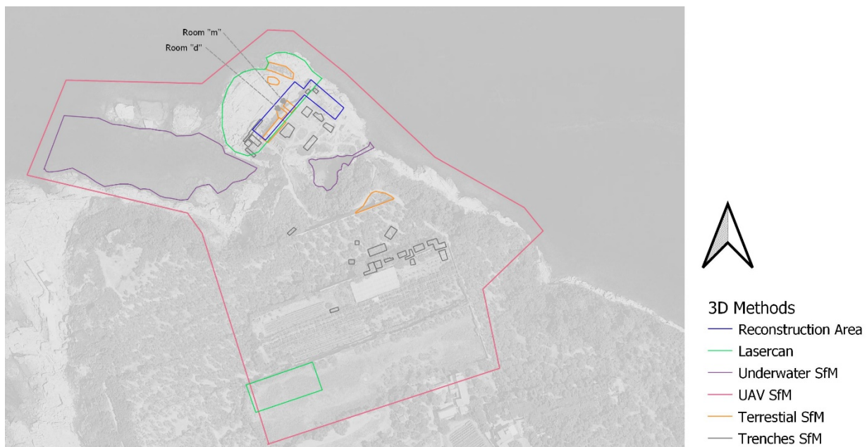
Figure 21. Overview of used methods of 3D documentation and reconstruction [B. Fritsch].
