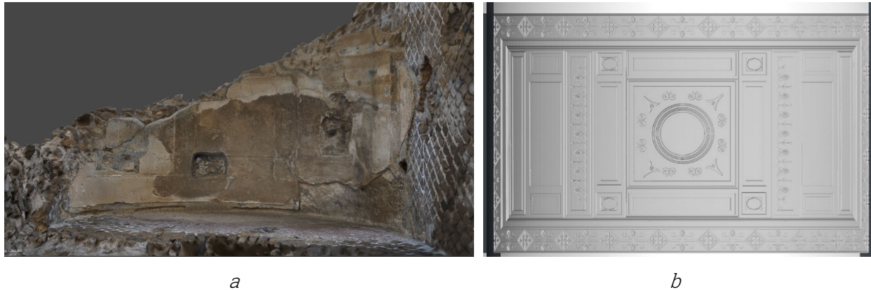
Figure 14. Screenshots of a) the SfM model of the stucco ceiling of the vault b) the partially reconstructed stucco ceiling [S. Götz]
