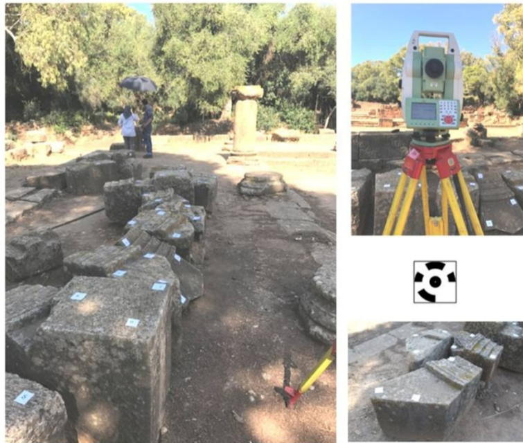
Figure 3. Use of the Total Station (Leica Total Station ST 11) for the survey of the targets placed on the stone blocks (a minimum of three targets is necessary to generate orthophotos at a later stage).
