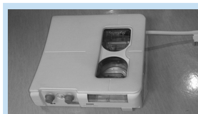
Fig.1. Breast coil used at Inkosi Albert Luthuli Hospital. Both breasts can be imaged simultaneously in the prone position.
