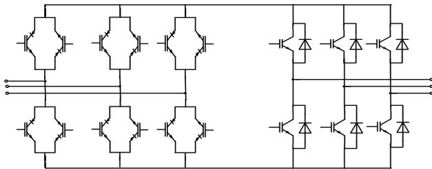
Fig. 9. Matrix converter or rectifier unit switches are based on RB-IGBT
