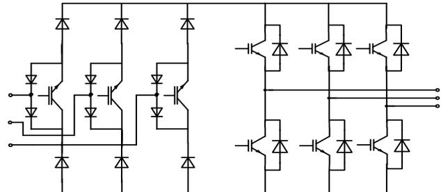
Fig. 7. Ultra-Sparse matrix converter
