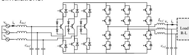
Fig. 11. Three-level Sparse Matrix Converter
