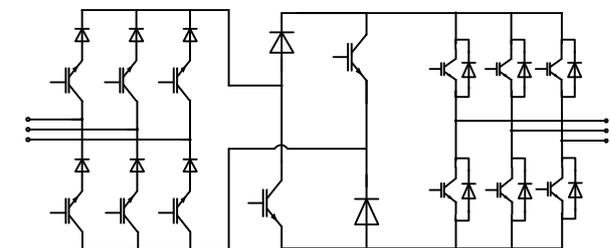
Fig. 8. Matrix converter with rectifier stage
