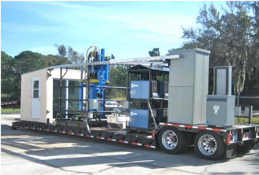
Figure 25: A picture of the 300 kW mobile magnegas refinery built by Santilli when Chief Scientist of Magnegas Corporation (now Taronis Corporation) to process a mixture of fossil oil and water into magnegas whose combustion with the proper stoichiometric oxygen has no detectable CO or HC [57]. The oxygen content of magnegas appears to have special polarizations [62] - [65] deserving tests for its possible use in ventilators to kill Corona viruses due to the emission of strong UV light in its depolarization in human lungs.
