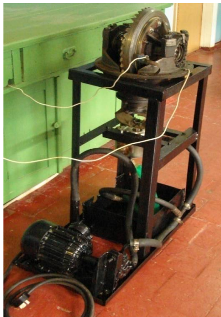
Fig. 3. General view of the installation for the implementation of technological processes of running-in methods of the gearing of the main transmission T-150K tractor
