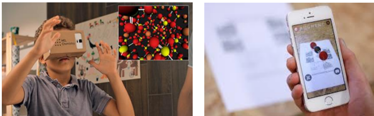
Figure 2. These images depict the VR and AR aspects of the VR/AR/WBVE system. The first image from the shows a cardboard headset that the mobile phones were inserted into, and the top right of that image shows an example of what students saw (in our case the students experienced only one molecule in the virtual environment). The second image depicts a molecule augmented onto a physical surface (very similar to what students experienced). WBVE consisted of a molecule on a phone screen that could be manipulated by swiping the screen.
