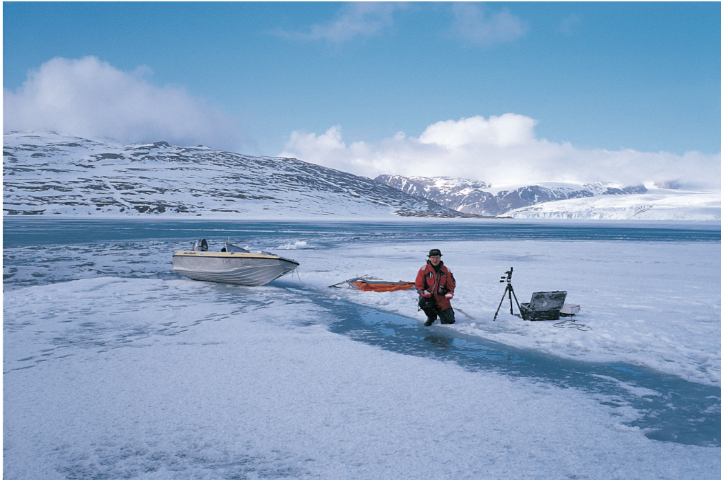
Study of the sea ice edge presents many challenges to researchers, particularly when in situ measurements are needed. Here, a scientist sets up a spectroradiometer to measure the reflectance of snow- and ice-covered surfaces in Kongsfjorden, Svalbard. (Photo S. Gerland, Norwegian Polar Institute Picture Library.)
