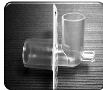
Figure 1. The Airway Breathing Circuit (ABC) elbow was cut before the angle so that a cylinder is produced.
