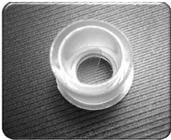
Figure 5. A circular acetate flap was positioned with the small tongue extension wedged between the cylinder and the ring
