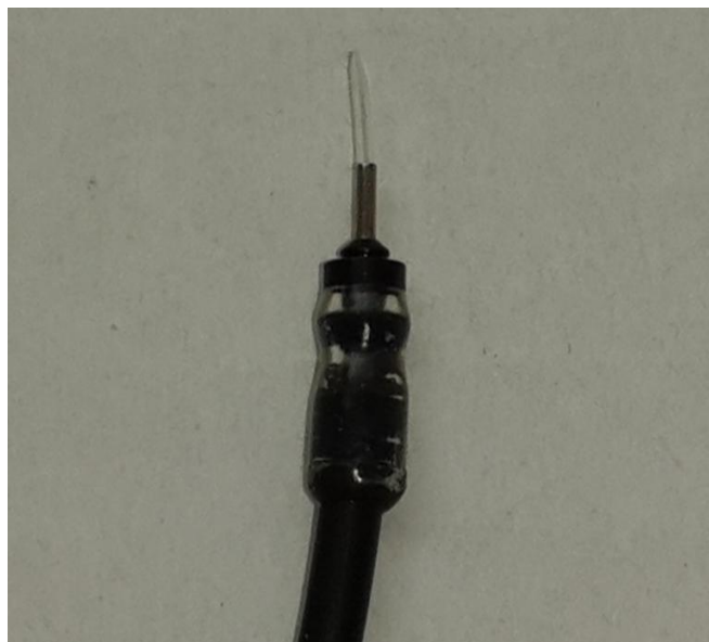
Fig. 2. Self retaining custom modified 23 G Endo Illuminator.
