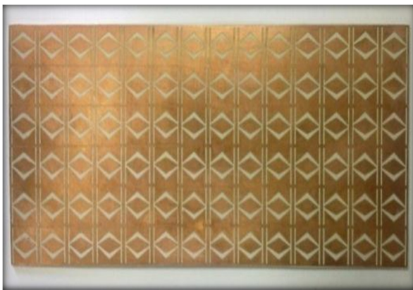
Fig. 7 An intermittent arrangement of base cells at 5 GHz
