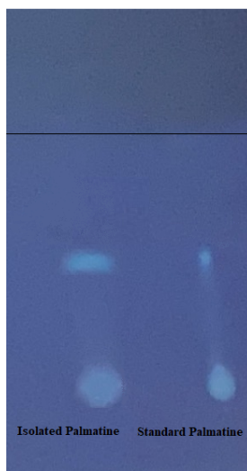
Figure 1. TLC of isolated palmatine compared to standard palmatine
