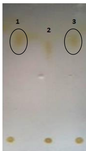
Fig. 5. Thin layer chromatography analysis of the EPS isolated from the strain CMS. The sample was placed on silica gel coated plates and the solvent system used was benzene, acetic acid and methanol (1 : 1 : 3).
