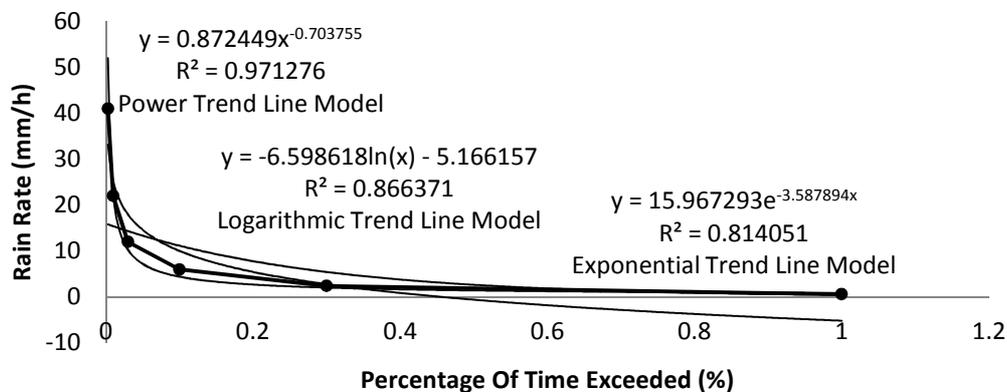
**Figure 1. The Graph Of ITU Rain Rate and Percentage of Time Exceeded for Rain Zone E.**
