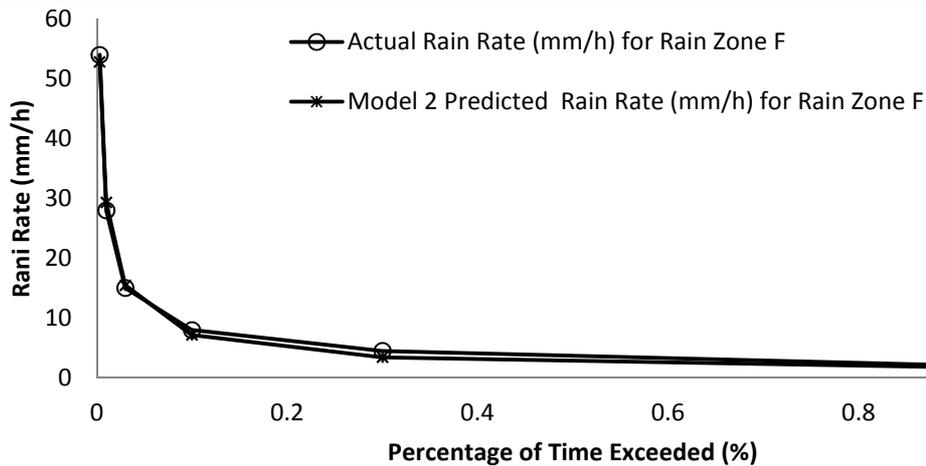
**Fig. 3 The Actual and Model 2 Predicted Rain Rate For Rain Zone F**
