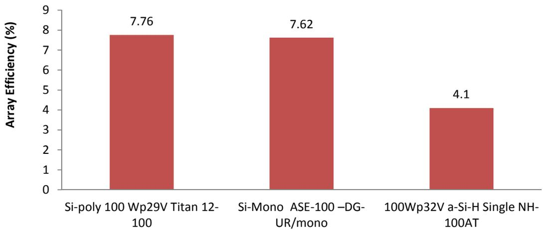
**Figure 4** Array Efficiency (%) for the Three PV Technologies
