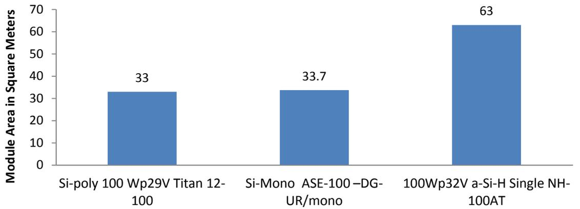
**Figure 3** Module Area in Square Meters for the Three PV Technologies
