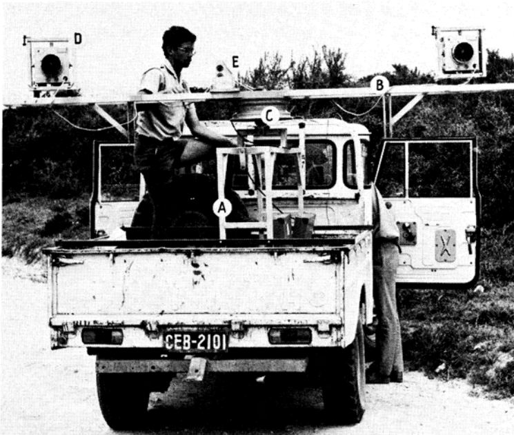
Fig. 2: A pair of UMK stereo cameras set up for simultaneous operation on a revolving mount which is secured on the back of a light truck: A– base frame; B– camera carriage frame; C– revolving hub; D– camera box; E– electrical trigger mechanism.
