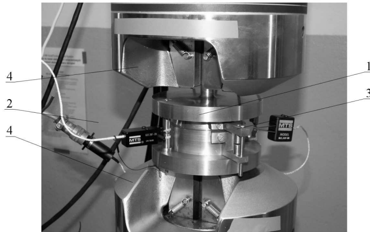
Fig. 14. The mode of fixing the model and an overview of its components: 1 – tested model, 2 – first extensometer, 3 – second extensometer, 4 – gripping jaws of an MTS testing machine
