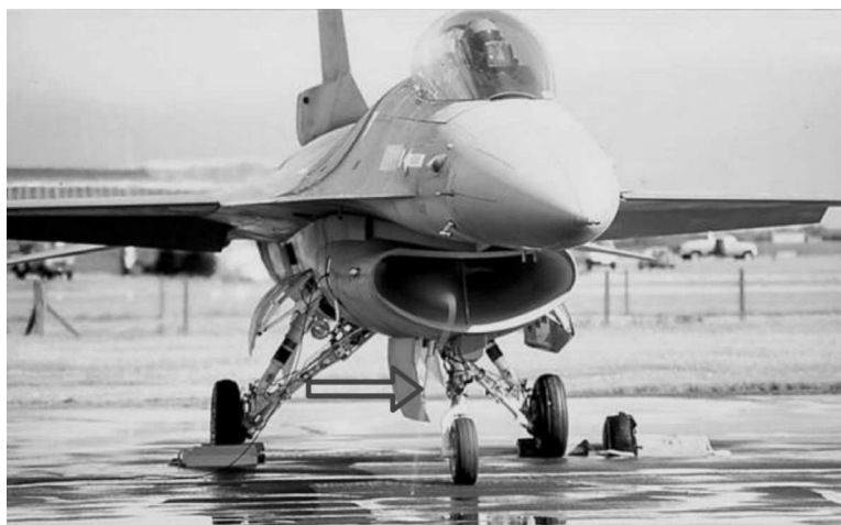
Fig. 4. An inlet vortex formed at F-16's inlet (indicated with the arrow)
