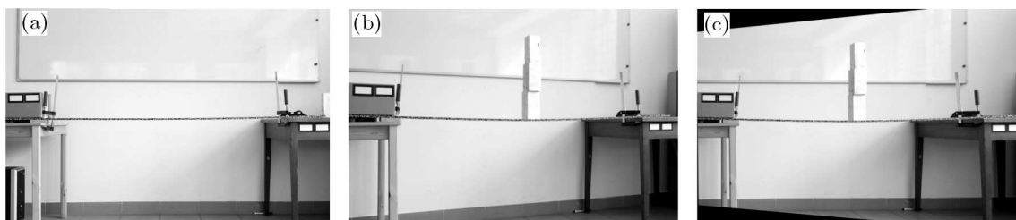
Fig. 2. (a) Reference image of the unloaded structure, (b) image of the loaded frame captured with projective distortions; (c) image rectified by the homography matrix computed from coplanar rectangular markers
