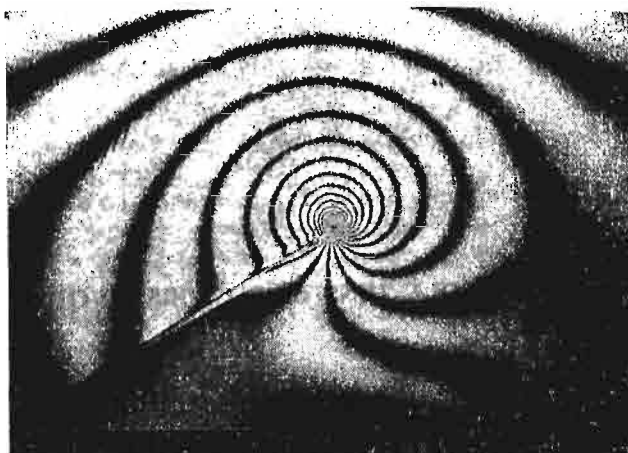
Fig. 1. Interference pattern of isopachics in the vicinity of the angled crack in a bend specimen
