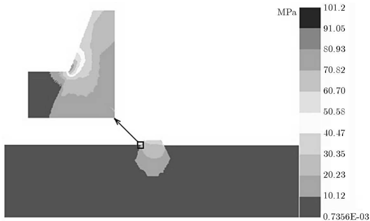
Fig. 6. Equivalent stress distribution on the diamond and the composite matrix
