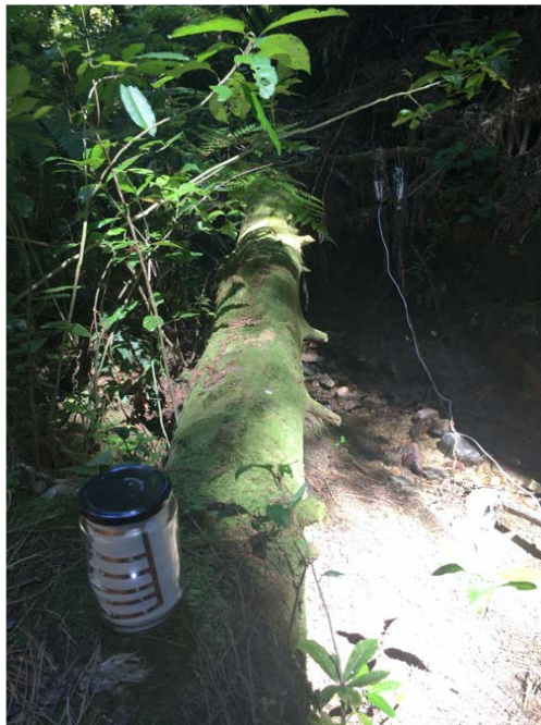
Figure 6: Papawai Stream installation showing visualisation node for electric conductivity in the front and sensors installed in the back
