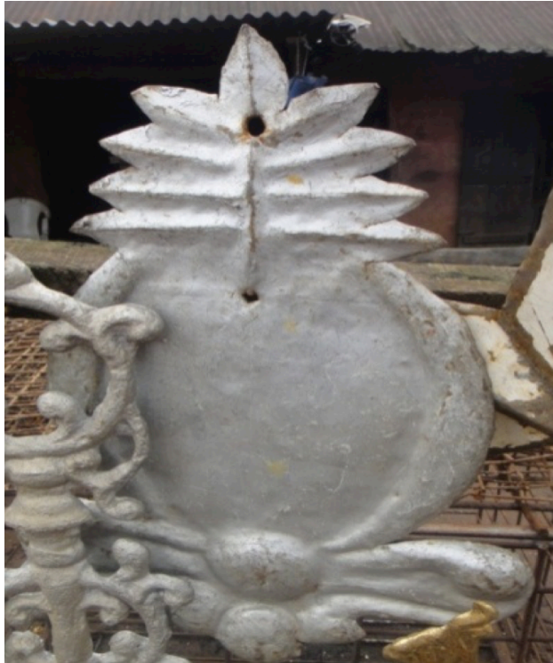
Figure 10 | A carbon steel floral shield rendered in chasing and repousse working technology (called beating by the blacksmiths). Photograph by Kingsley O. Emeriewen, 2012.
