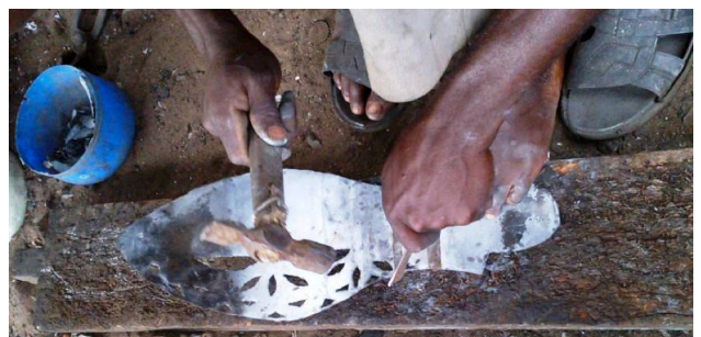
Figure 7 | Cutting out traced patterns on a traditional sword with a chisel made from carbon steel strip. Photograph by Kingsley O. Emeriewen, 2013.
