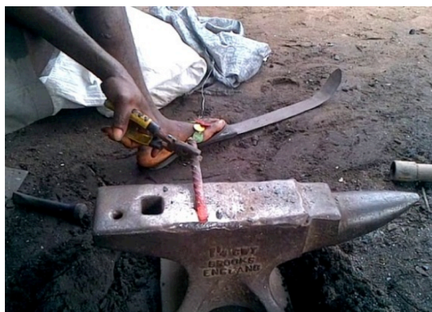
Figure 9 | Hammering a red-hot steel rod to form a spike. Photograph by Kingsley O. Emeriewen, 2013.
