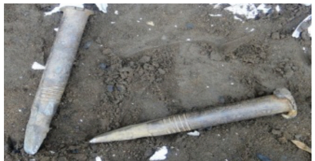
Figure 6 | Variants of pritchels (for creating holes). Photograph by Kingsley O. Emeriewen, 2012.
