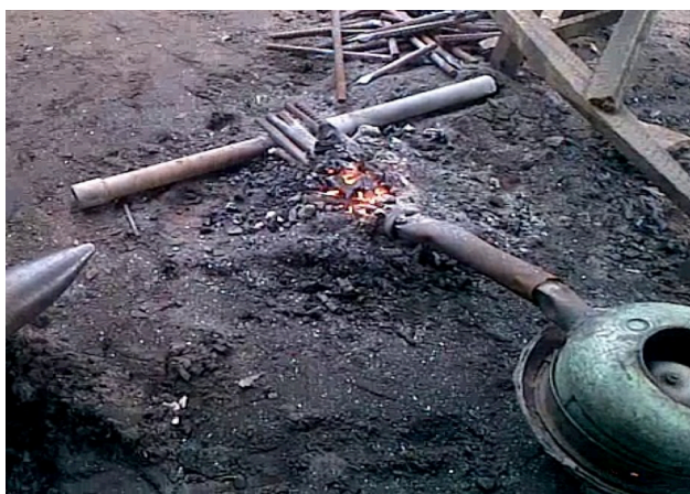
Figure 8 | Firing carbon steel rods in a furnace. Photograph by Kingsley O. Emeriewen, 2013.
