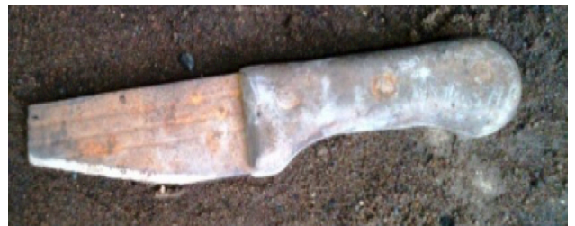
Figure 5 | A cutlass improvised as chisel for cutting. Photograph by Kingsley O. Emeriewen, 2012.
