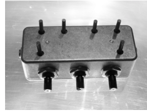
Figure 4 | The bi-core unit, left potentiometer controls on-time of the LED, right potentiometer the off- time.
