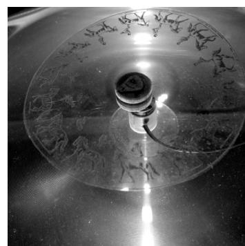
Figure 5 | The Picture-disc is mounted on a dc-motor. The motor is fixated with a vacuum cup on the screen.
