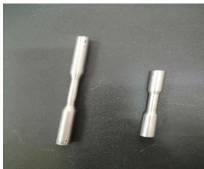
Figure 5. Tensile test specimen dimensions
