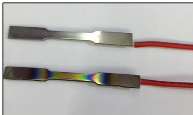
Figure 2. Coated and uncoated work substrate before covering
