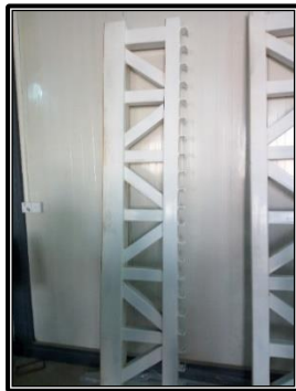
Figure 4 Cast of CFST truss girder.
