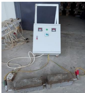
Figure4. Corrosion test method
