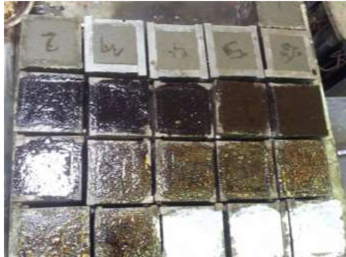
Figure (2): covering the specimens with curing solutions after 30min of casting
