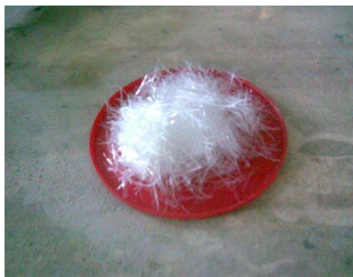
Figure 2 Polypropylene fiber configuration that is used in this study.
