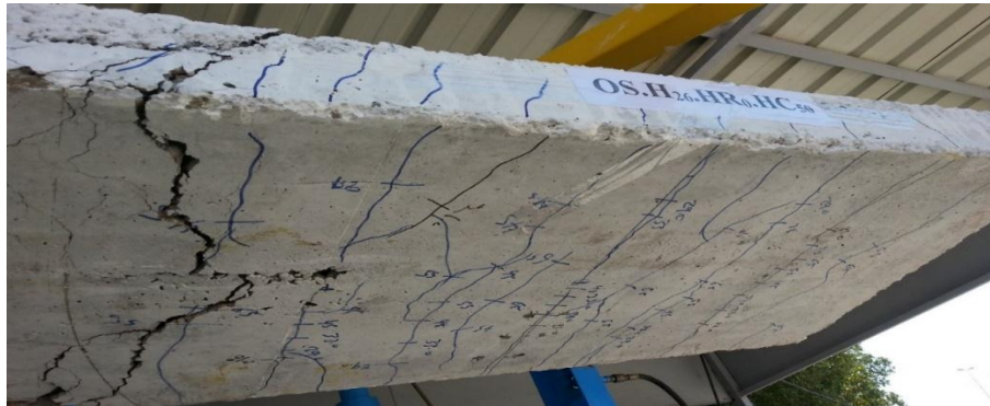
Plate 2 Mode of Failure and Cracks Pattern of Specimen OS.H26.HR0.HC25
