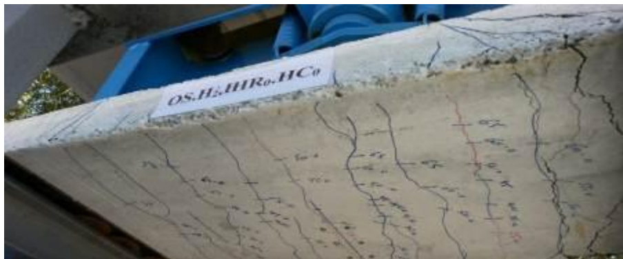
Plate 1 Mode of Failure and Cracks Pattern of Specimen OS.H26.HR0.HC0
