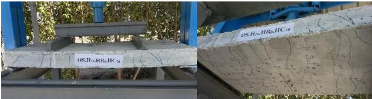
Plate 4 Mode of Failure and Cracks Pattern of Specimen OS.H26.HR0.HC75
