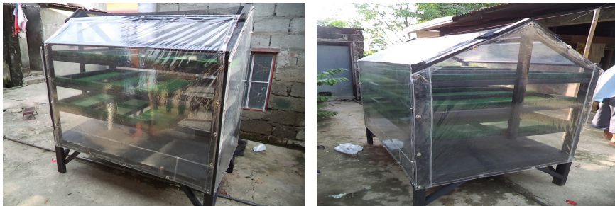
Figure 7 and 8. The actual view of the fish dryer natural convection facility
