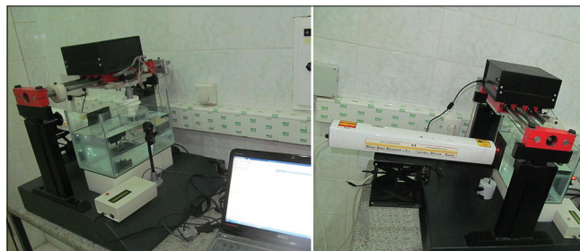
Figure 5: Designed and constructed optical computed tomography system
