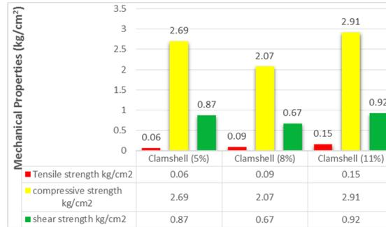
Fig. 2. Mechanical Properties Analysis Sand Moulding in Dry Conditions
