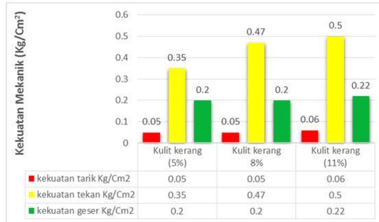
Fig. 3. Mechanical Properties Analysis of Sand Moulding in Wet Condition
