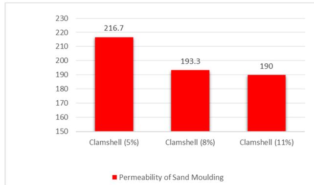
Fig. 4. Bar chart Sand Mould Permeability Testing Results of the variety of shells
